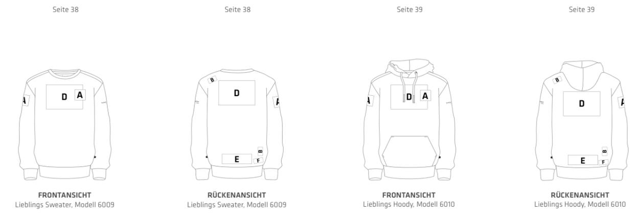
A = 70x70mm    B = 70x40mm    C = 90x120mm    D = 240x160mm    E = 210x70mm    F = 80x40mm    G = 70x25mm    H = 60x200mm
